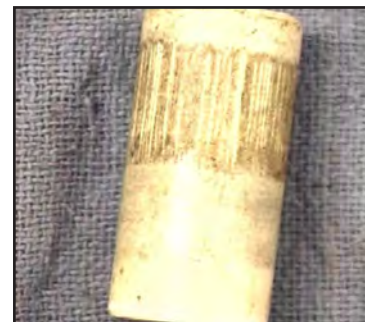
Figure 5-8. Examine Ceramic Plungers
