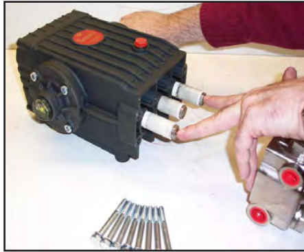
Figure 5-16. Re-install Manifold and Torque Fasteners
