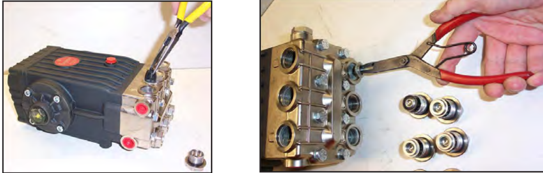
Figure 5-1. Remove Valve Cap and Valve Assembly
