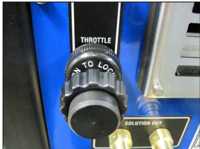
Figure 4-4. Turn Throttle Cable Knob Counterclockwise to Increase
